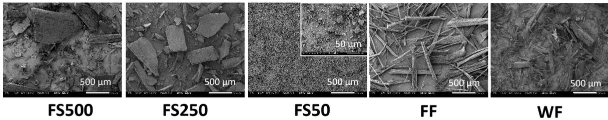
Figure 2. Length distribution of reinforcing materials and visual aspect as observed with SEM.
