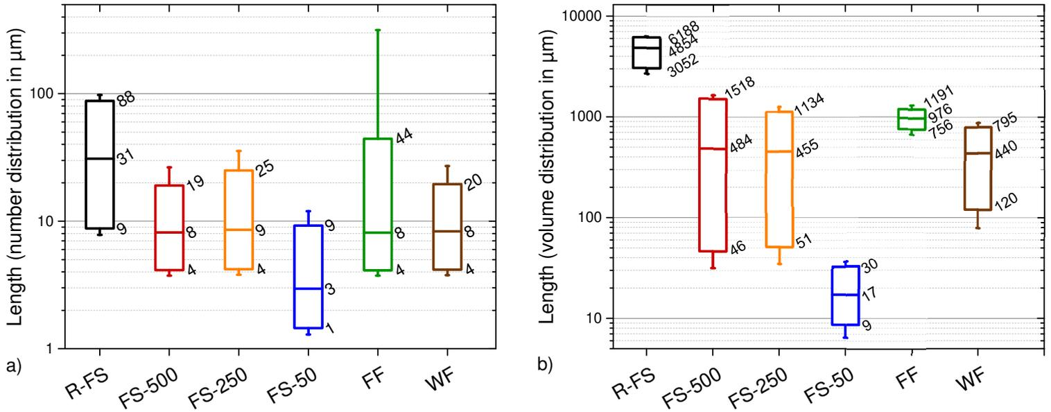
Figure 1. Reinforcing material length distribution after comminution a) in number, b) in volume. The 10<sup>th</sup> (first decile), 16<sup>th</sup>, 50<sup>th</sup> (median), 84<sup>th</sup>, and 90<sup>th</sup> (last decile) percentiles of the cumulative distribution in length are shown respectively from bottom up with corresponding values of 16<sup>th</sup>, 50<sup>th</sup> and 84<sup>th</sup> percentiles facing them.
