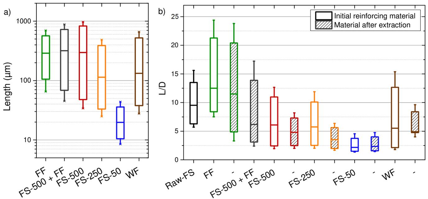
Figure 6. a) Particle length distribution in volume and b) Aspect ratios of *initial reinforcing material compared to extracted materials from the 30%-wt reinforced PP-MAPP composite*. The 10<sup>th</sup> (first decile), 16<sup>th</sup>, 50<sup>th</sup> (median), 84<sup>th</sup>, and 90<sup>th</sup> (last decile) percentiles of the cumulative distribution in length are shown respectively from bottom up.
