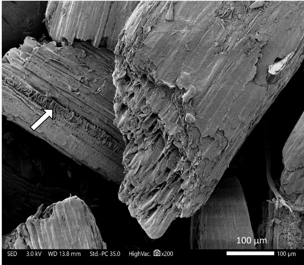
*Figure 3. Preserved cell wall alveolar structure of some FS-250 particles after comminution. Arrow points to an interesting tracheary element of the flax xylem.*
