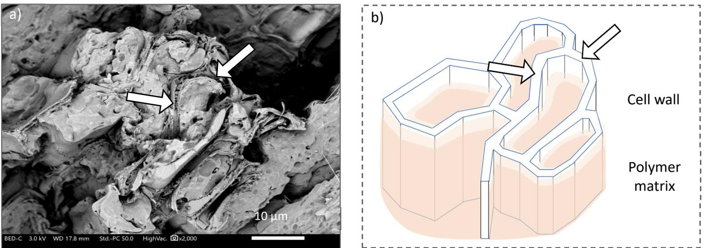
Figure 11. a) SEM observation of the fracture surface of the 30%-wt FS-500 reinforced PP-MAPP composite b) Highlight of a potential matrix penetration in the alveolar structure. Arrows indicate cell-walls.
