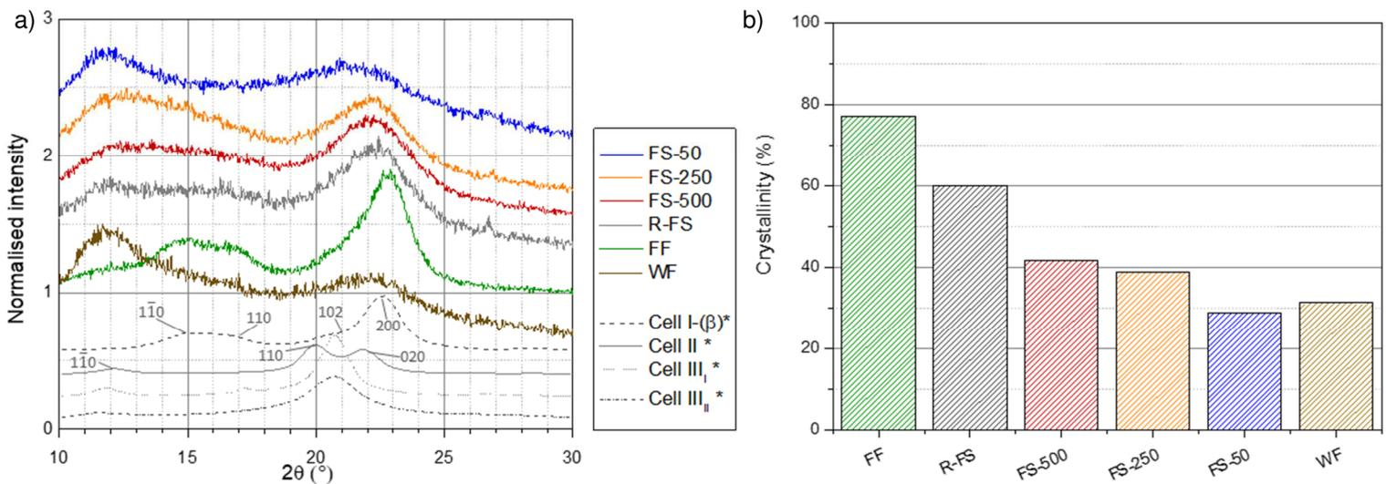
Figure 5. a) XRD spectra for the **fragmented** flax shives (raw, 50, 250, 500). For reference, the XRD spectra of Avicel cellulose from Lee et al. [49] marked with \* on the graph are also illustrated. b) The evolution in the crystallinity of the samples.
