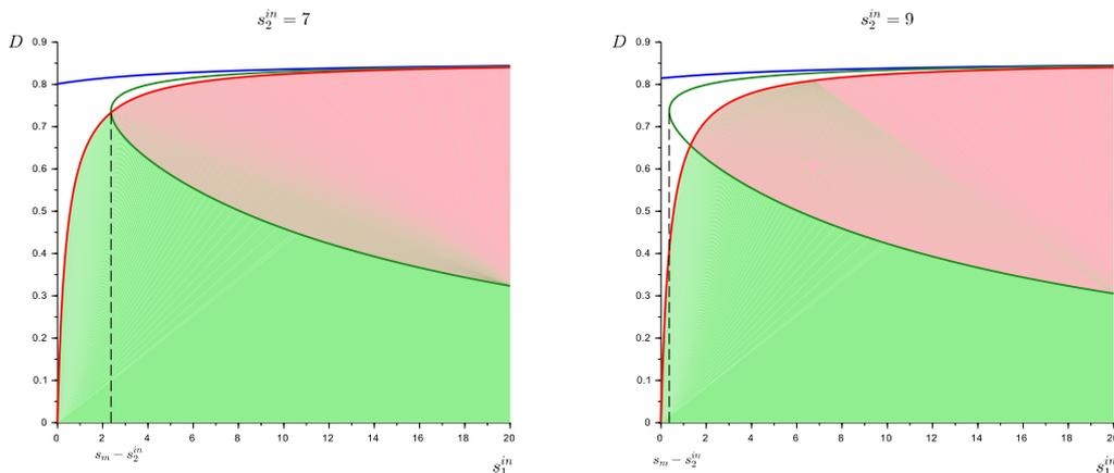
Fig. 5. Cross-sections of the domains  $\mathcal{D}_5$  and  $\mathcal{D}_6$  for  $s_2^{in} = 7$  and  $s_2^{in} = 9$ . From any operating point  $(s_1^{in}, D) \in \mathcal{C}_5$  it is not possible to reach  $\mathcal{C}_6$  by simply increasing  $D$ .
