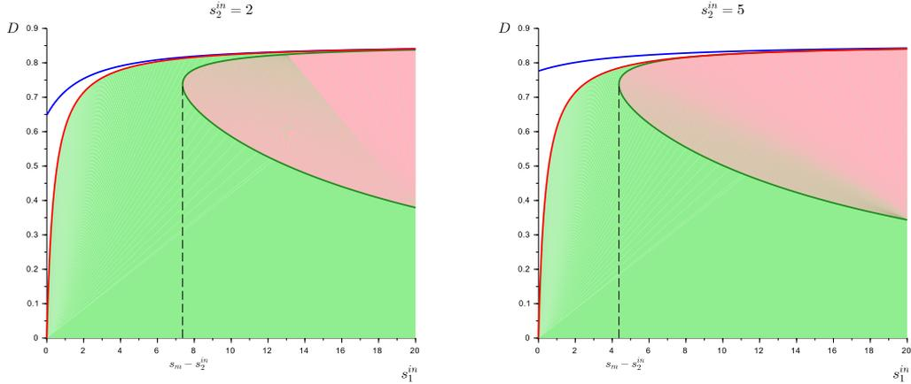
Fig. 4. Cross-sections of the domains  $\mathcal{D}_5$  and  $\mathcal{D}_6$  for  $s_2^{in} = 2$  and  $s_2^{in} = 5$ . From an operating point  $(s_1^{in}, D) \in \mathcal{C}_5$  with  $s_1^{in}$  not too far from  $s_m - s_2^{in}$ , it is possible to reach  $\mathcal{C}_6$  by simply increasing  $D$ .
