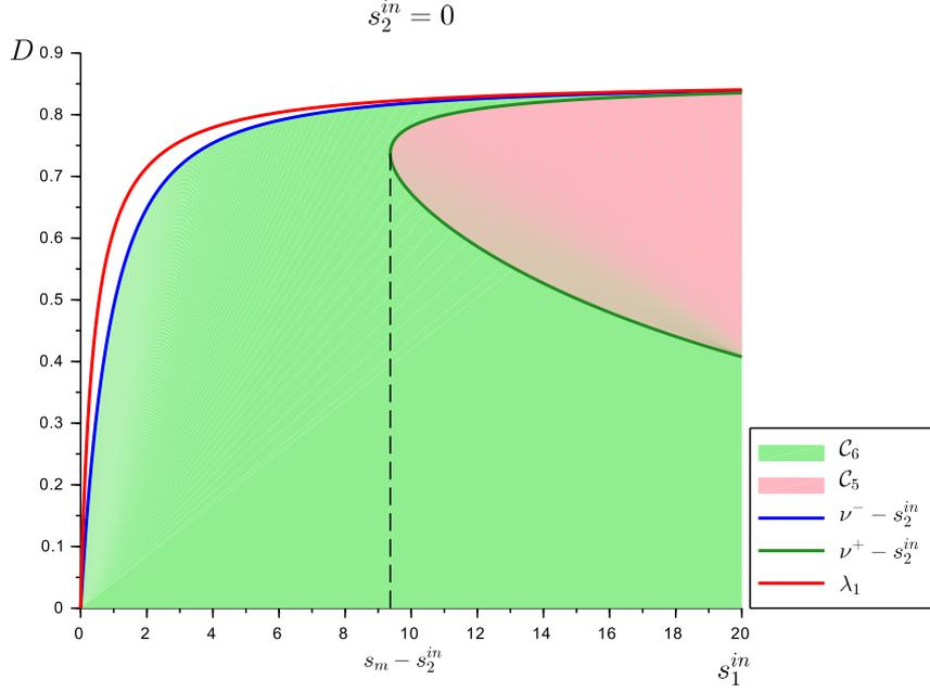
Fig. 3. Cross-sections of the domains  $\mathcal{D}_5$  and  $\mathcal{D}_6$  for  $s_2^{in} = 0$ . From any operating point  $(s_1^{in}, D) \in \mathcal{C}_5$  it is possible to reach  $\mathcal{C}_6$  by simply increasing  $D$ .
