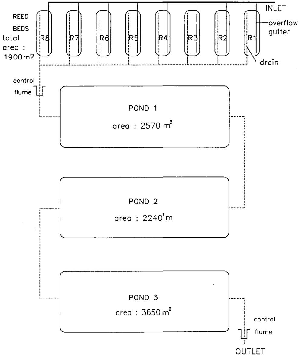
Fig. 4. Schematic description of the Gensac plant.
