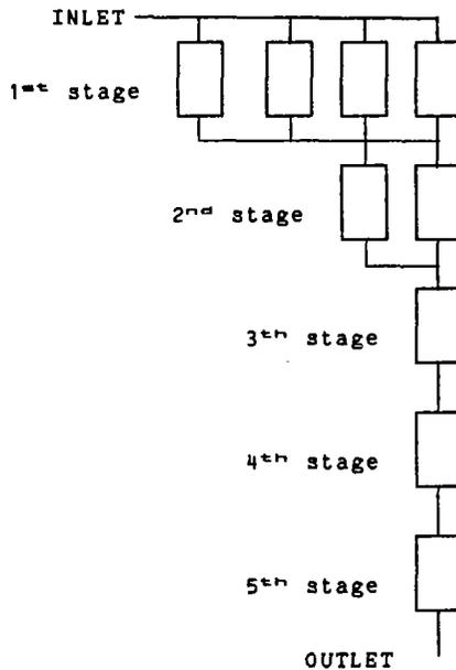
Fig. 1. Typical layout of a MPIP plant
