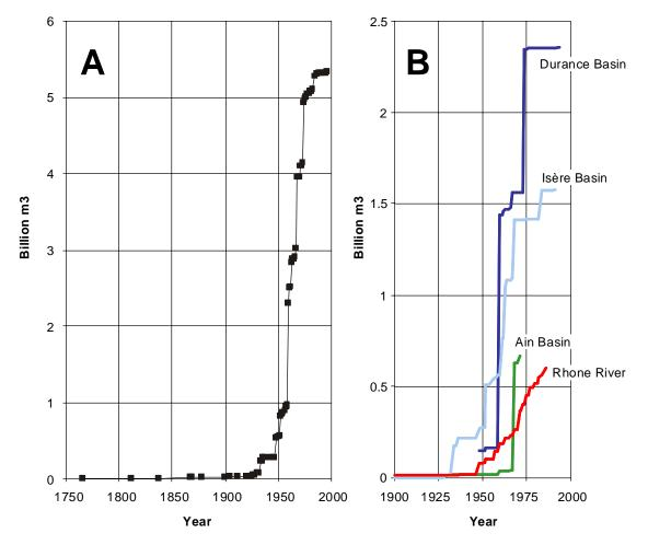
Fig. 3. Cumulative reservoir capacity of dams with a height of 15 metres or more. (A) All the dams of the French Rhone Basin. (B) Dams of the main tributary catchments (Durance, Isère and Ain Basins) and of the Rhone itself which significantly contribute to water storage in the basin. Data from the database of the International Commission on Large Dams (ICOLD, 2002).
