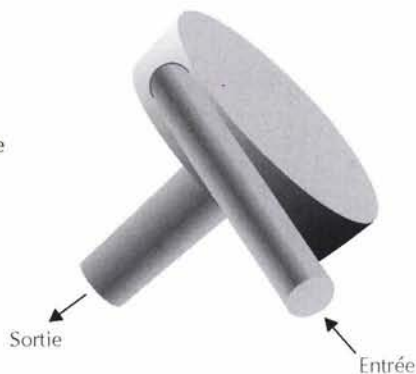
Figure 3.6 – Principe de la diode hydraulique
