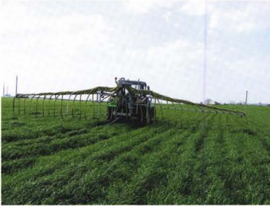
Photo 3.4 – Épandage sans tonne [F. Thirion, Cemagref]
