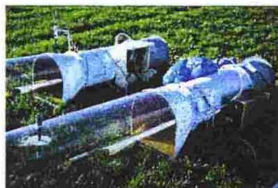
Tunnels de ventilation sur prairie Wind tunnels on grassland (Scaër, mars/march 1993)
