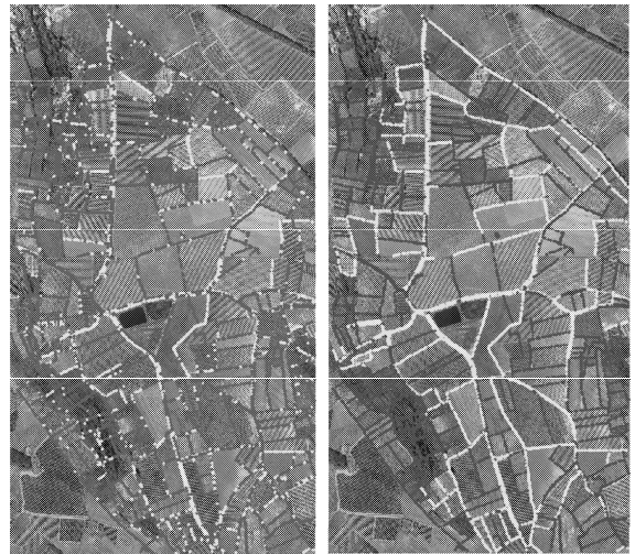
FIG. 6 – Comparison between classification of ditches presence (light grey) on the left and ground truth data on the right for each plot boundary location on the 2\text{km}^2 test area
