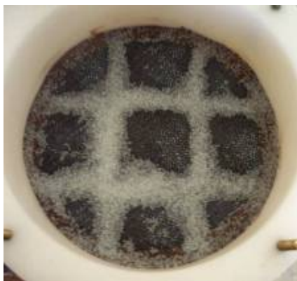
Figure 7. Illustration of the use of glass beads to reach a flat surface on top of the GCL samples
