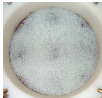
Figure 7. Illustration of the use of glass beads to reach a flat surface on top of the GCL samples
