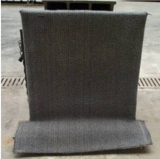
Figure 3. Piece of GCL1 before testing in the heavy rainfalls situation.
