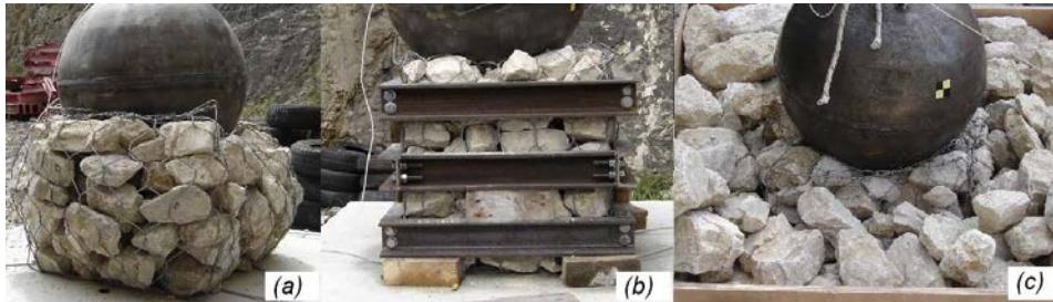
Figure 4. Lateral boundary conditions used in the experiments: a) free-to-deform (FD) ; b) rigid confinement (RC) ; c) material confined (MC) (after Lambert et al., 2009).
