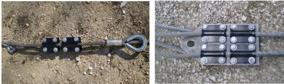
Figure.5. 2 steel plates 1 for SB device (left) - Longer steel plate 2 for MB device (right)
