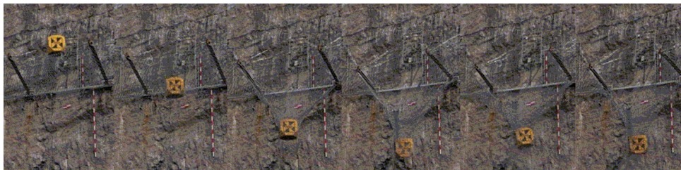
Figure.14. Sequence impact 16000kg block to 25m/s h=32m vertical test tested in Walenstadt during 2006. Barrier type RXI-500 (5000kJ)
