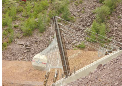
Figure.4. 3000 kJ impact on the new test site
