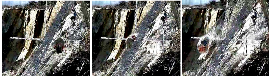
Figure.4. a) boulder before horizontal impact c) first impact d) maximum net deflection
