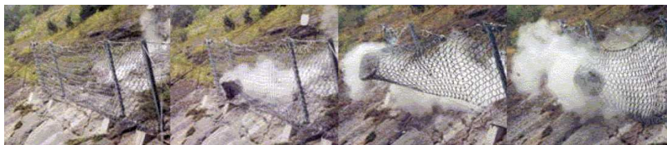
Figure.13. Sequence impact 5600kg block to 27m/s inclined cable car tested in Beckenried during 1997. Barrier type RX-200 (2000kJ)
