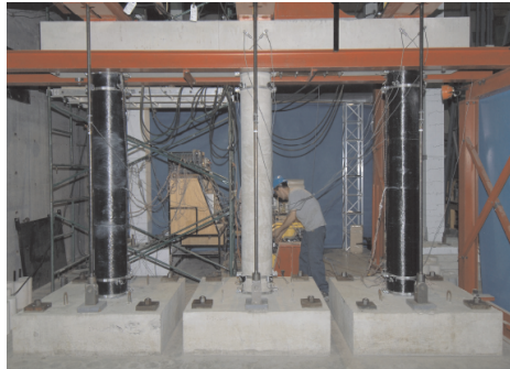
Figure 3. Bridge pier mockup with partial retrofitting.
