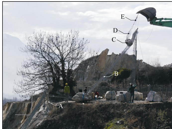
Figure.3. Cross sectional view of test site and apparatus. [A] Test hybrid barrier with impact zone at top [B] Release ramp constructed of SPIDER wire net [C] Natural test boulder [D] Release nets constructed of snow net [E] Automated remote release hook
