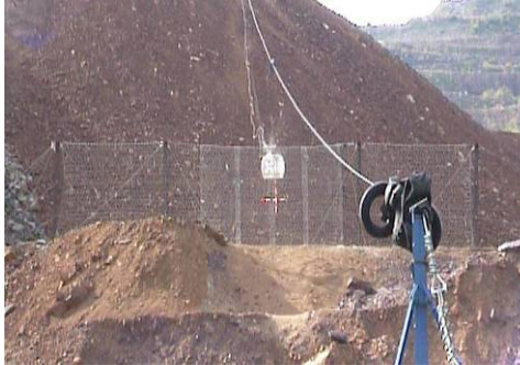
Figure.3. Full scale test at the test site Erzberg using the first cable car
