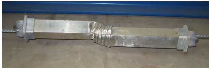
Figure.7. Progressive buckling of an aluminum dissipator
