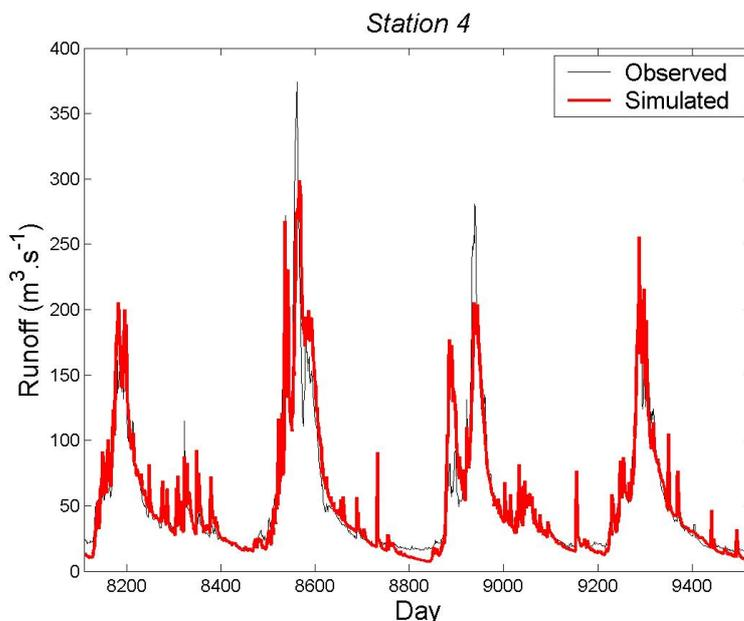
Figure 6. Illustration of SIM-generated runoff vs. observed runoff.
