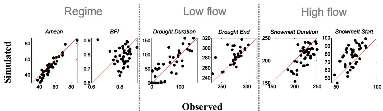
Figure 7. Comparison of selected hydrologic indices computed for observed and simulated streamflow.
