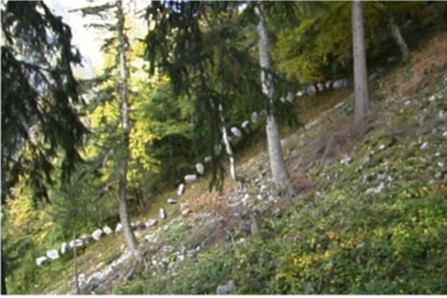
Figure 2. Rebound of a rock reconstructed from a series of successive images extracted from a camera film (50 frames per second). This figure is available in colour online at wileyonlinelibrary.com/journal/espl
