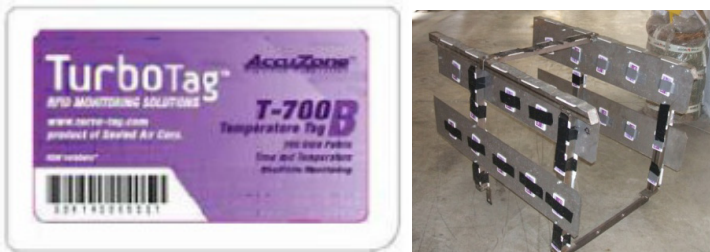
Fig.2. Turbo Tag ® card and framework with all Turbo Tag ® cards installed
