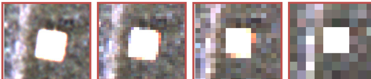
Fig. 7. Example of transformed images at different spatial resolutions: 1.8, 5.3, 10.7 and 19.9 cm, from left to right respectively
