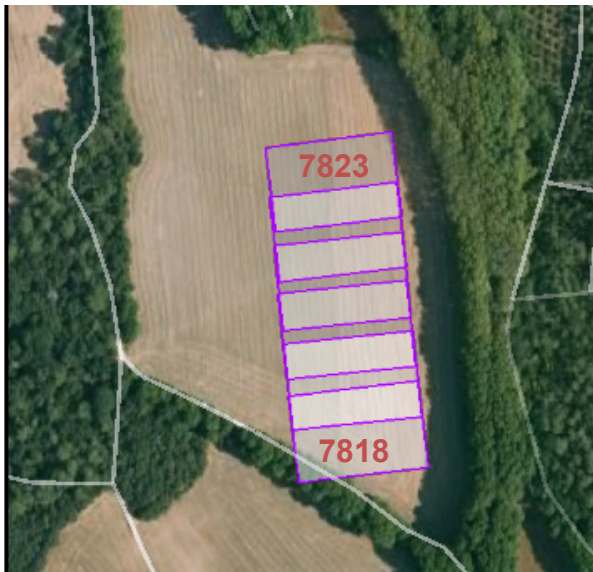
Fig. 6. Sequence of six images (numbered from 7818 to 7823) taken at Castries. Image contours are marked in purple and image overlapping in white
