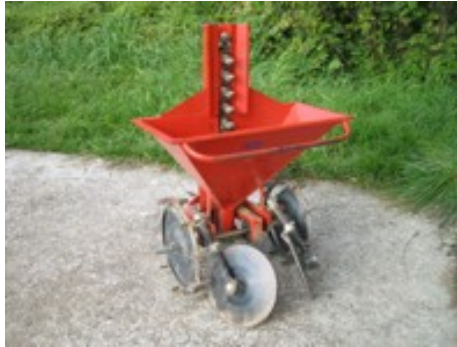
Fig. 1. Modified single row potato planter used in the traditional farm system of Vessalico for planting garlic
