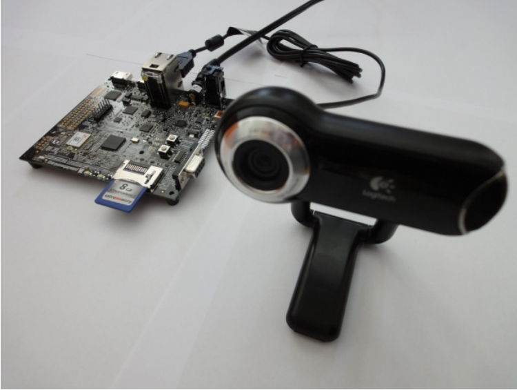
Fig. 1. SBC test setup. A Logitech USB camera is attached to the Board.
