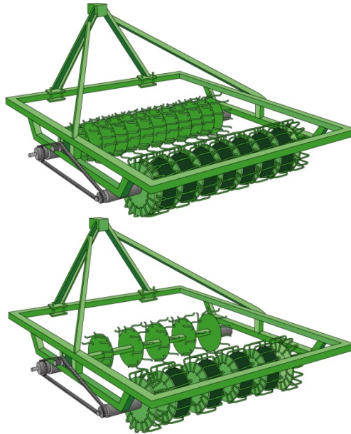
Fig. 3. The rolling harrow: close arrangement for full surface treatment (top); spaced arrangement for inter row treatment (down)
