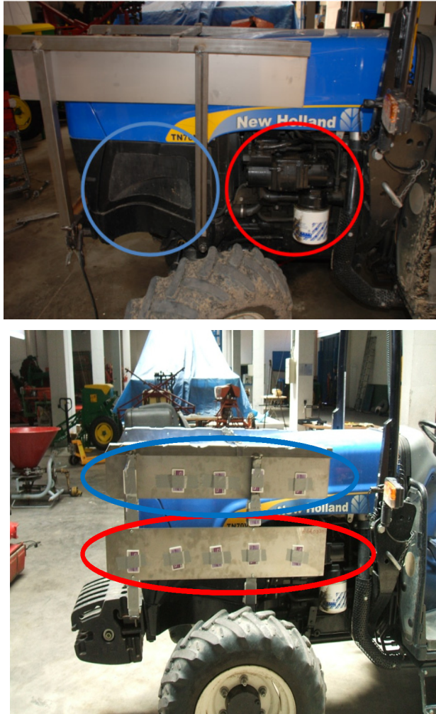
Fig.4.Engine air inlet (blue circumference), engine air outlet (red circumference) and longitudinal and height heat distribution (by red ellipse representing expected warmer places and by blue ellipse the least)
