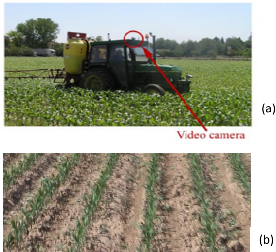
Fig. 1. (a) Position of the video camera on top of the tractor; (b) An example of a framer corded in the video.
