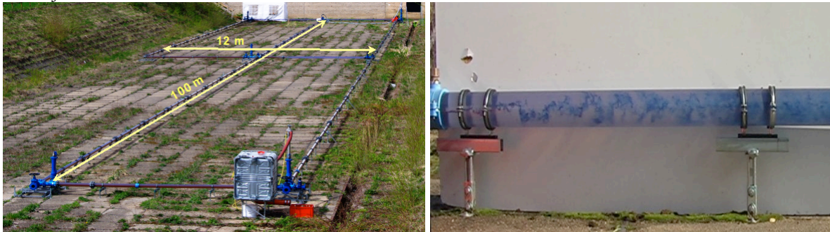
Figure 6: Test network for SMaRT-Online WDN (left); Injection experiments with a color tracer (right)
