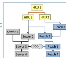
Figure 5: Routing in J2000P. Addition of a sewer network. Some SODs can connect sewer reaches to river reaches.
