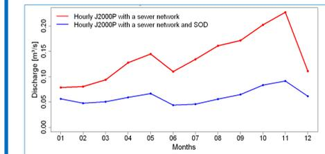
Figure 9: Mean interannual monthly sewer runoff at Taffignon between 1998 and 2010.
