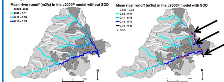
Figure 10: Mean river runoff between 1998 and 2010 simulated without or with SODs.
