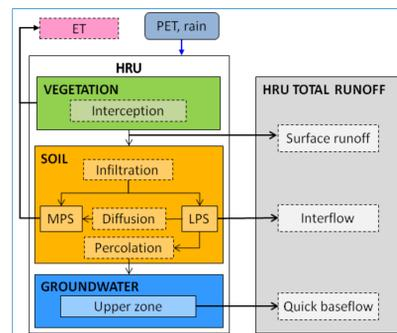
Figure 4: Physical processes and runoff contributions simulated at each time step and for each HRU.
