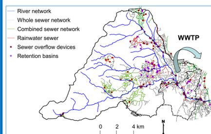
In urban areas: rainwater is mainly directed to the WWTP outside of the basin using combined sewer network (Fig.3).
