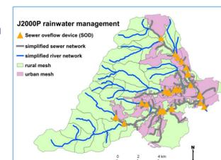
Figure 7: HRU delineation, sewer network and SODs.
