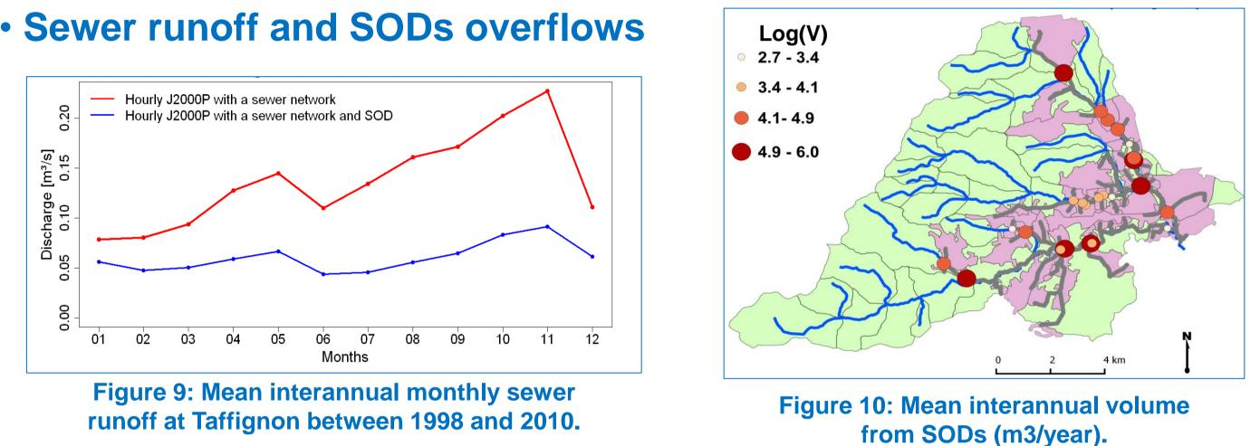
The sewer flow is affected by the presence of SOD (Fig.9). Overflows happen for almost all the SODs (Fig.10) and some can really impact the environment, especially during low flow periods.
