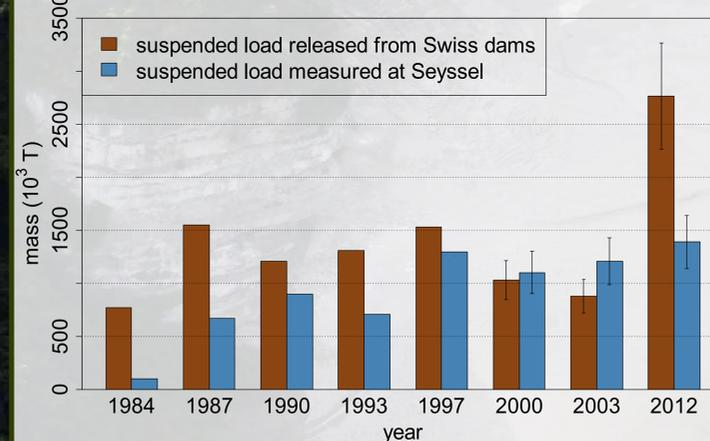
Figure 6 : Suspended load upstream and downstream of Génissiat reservoir [updated from Thareau, 2006]
