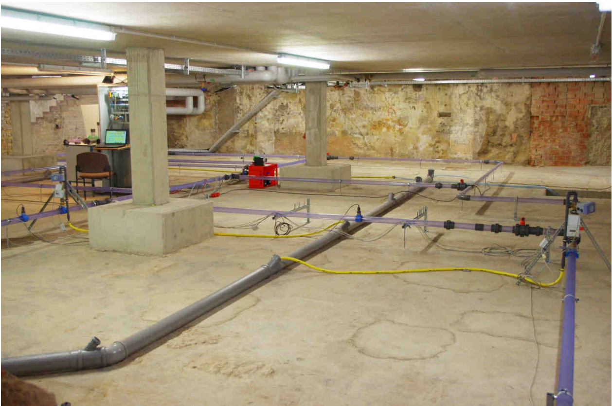
Figure 16: New indoor model network of TZW (Dresden)
