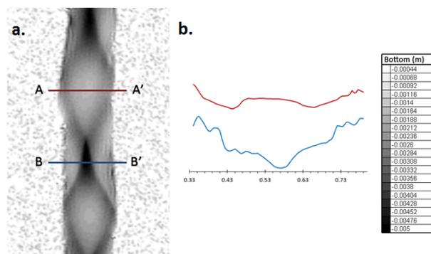
Figure 3.5: The formation of bars, a. the bed's topography (*Run 0*), b. cross section of the bed, in red the cross section of a bar and in blue the cross section of a scour hole
