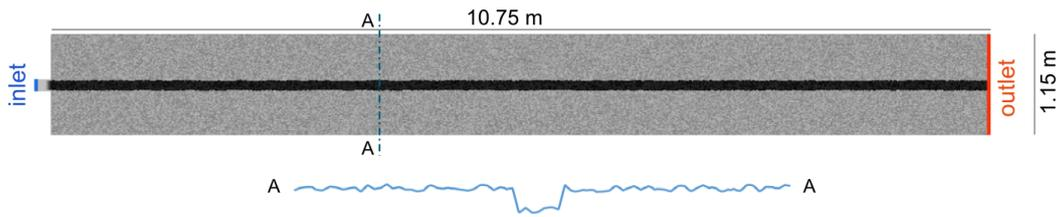
Figure 3.1: The geometry of the model, a. the dimensions of the model reminds the dimensions of a flume, b. detail of the unstructured mesh, c. cross section of the model
