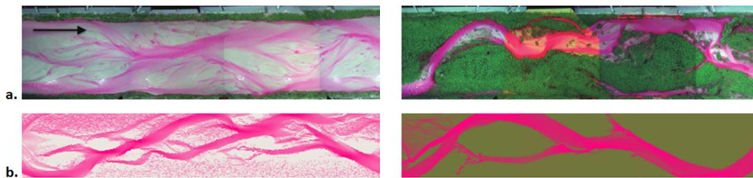
Figure 4.4: a. Transition from a braiding pattern to a single-thread channel caused by the vegetation of the floodplain (Tal and Paola, 2010), b. Similar transition observed in the *Run 02* (the choice of colors only serves illustrative purposes)
