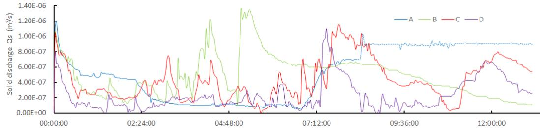
Figure 3.18: Evolution of the bedload rates at different transects ( *Run 01* starts at 02 : 15)
