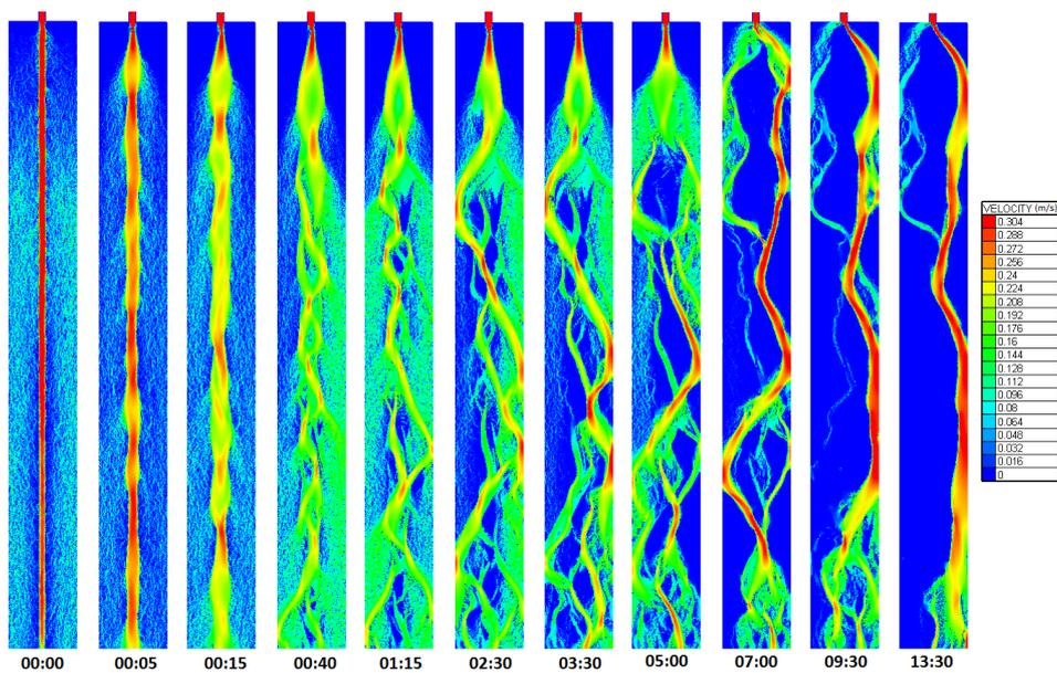
Figure C.2: *Run 0 – 00*: Flow velocity evolution through time
