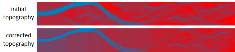
Figure 2.9: The adjustment of the bed topography, the dry areas are flattered
