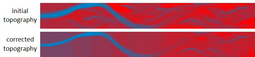
Figure 2.9: The adjustment of the bed topography, the dry areas are flattened
