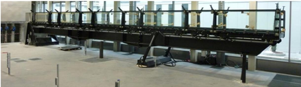
Figure 2: Canal inclinable IRSTEA-Lyon
