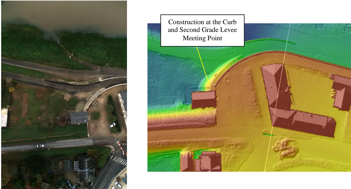
Figure 31: Example of a Transition between a Quay Wall, a House and an Earth Levee
