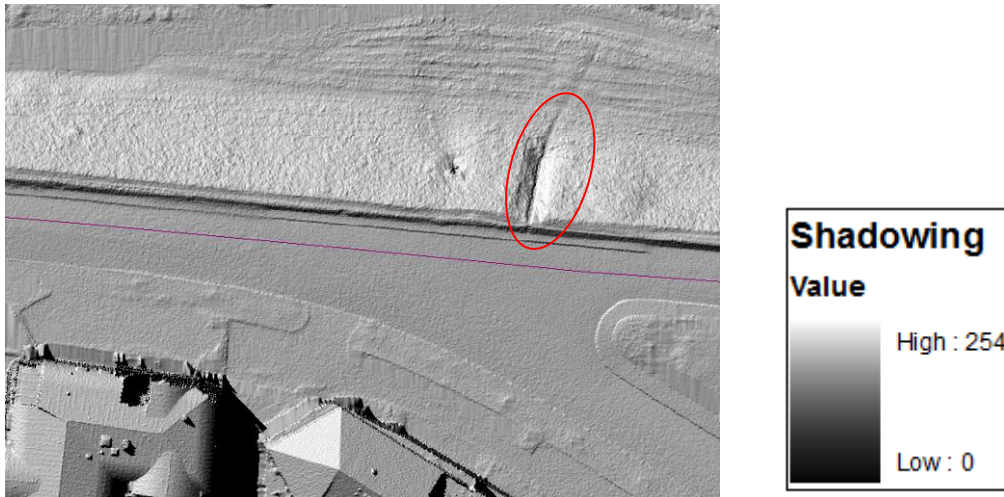
Figure 19: Shadowing Treatment on DSM
