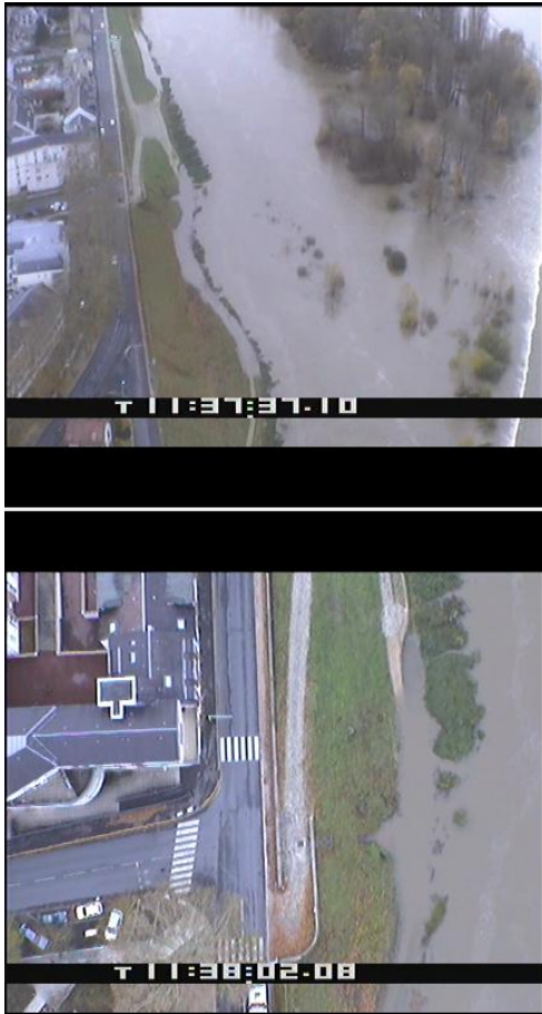
Figure 36: Oblique and Nadir Videos (Left) and Nadir Photograph (Right) of a Sample Levee with a Curb in Urban Area
