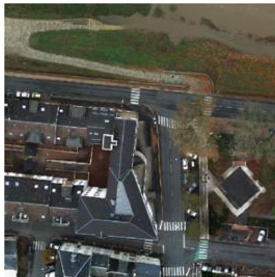
Figure 7: Example of Ortho-corrected Photograph (Produced from Raw Picture Pairs)
