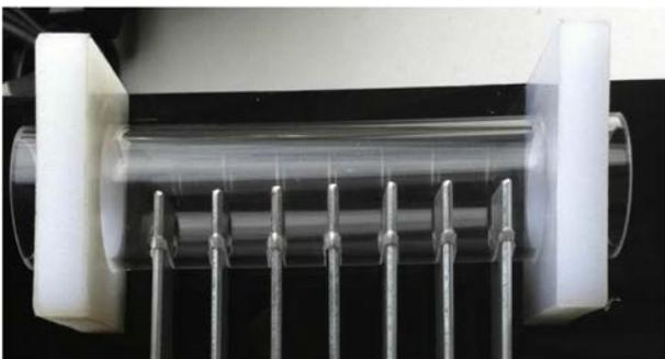
Fig. 3 – Connection between header and tubes.
