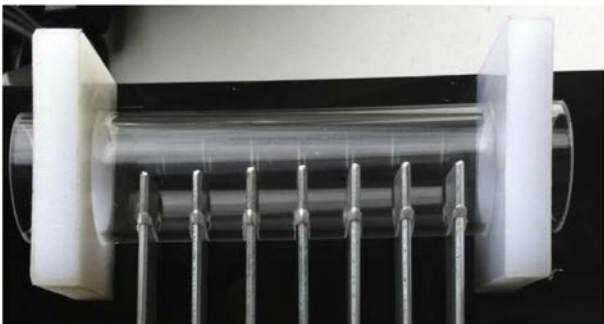
Fig. 3 – Connection between header and tubes.
