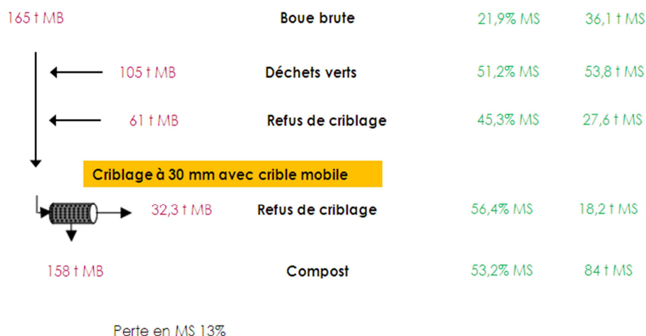
Figure 23: Bilan matière du site Es (compostage tunnel)
