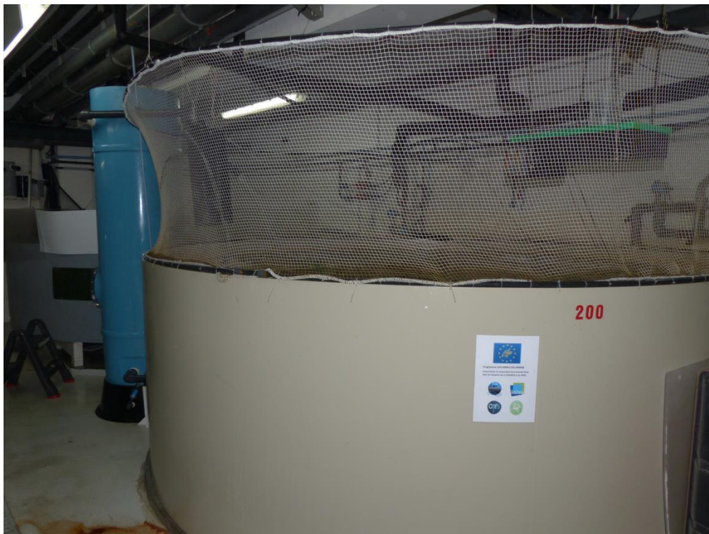
Figure 1: The 8 m 3 rearing tank with the new net to prevent escapements.
