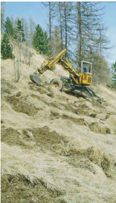
30. The mechanical "spider" digger, which digs planting holes in appropriate sites, enables foresters to plant saplings with covered roots under harsh conditions. This tool can reach steep slopes up to 60%.
