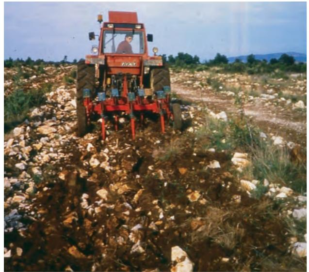
29. Subsoiling on rocky soils greatly improves establishment success and plantation start-up by accelerating root development. This operation is performed with 1 (left), 2 or 3 (right) teeth, depending on soil resistance and can be followed by a levelling operation.
