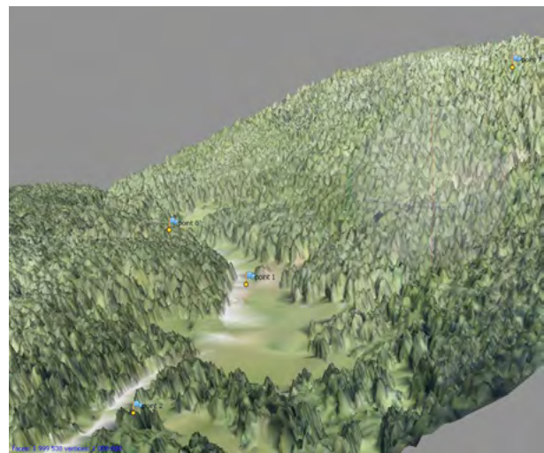
Figure 21: Results of a UAV-mission. Flight-path and image locations (Asiago test site) (left), 3D-model of the Asiago test site, constructed from 260 aerial images (right)
