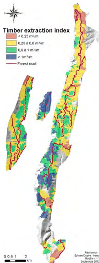
Figure 31: Map of the timber extraction index (total volume extracted on a single cable line divided by the length of this line). Areas with an index > 0.6 \text{ m}^3/\text{m} are potentially the most interesting for cable yarding operations
