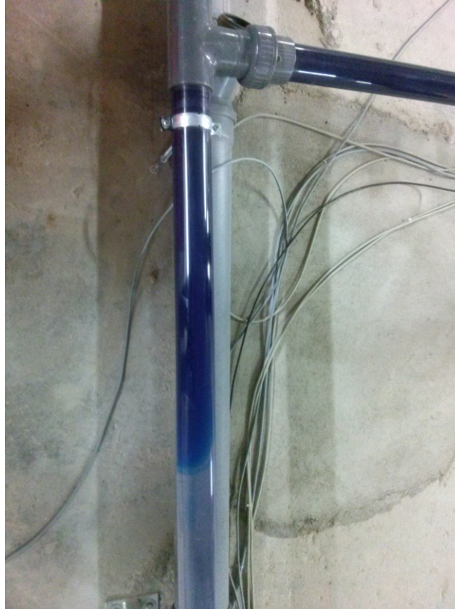
Figure 13: Contamination front (blue tracer colour)
