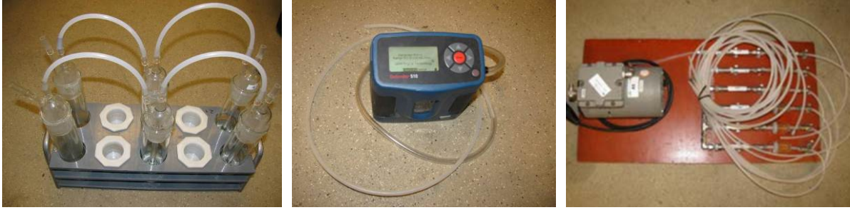
Figure 4. Set-up gas washing method. Left: acid traps. Middle: Flow meter. Right: pump
