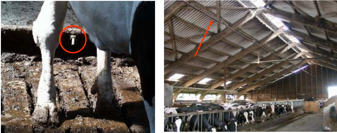
Figure 13. Tracer gas method in practice. Left: injection point; Right: sampling line with a number of sampling points
