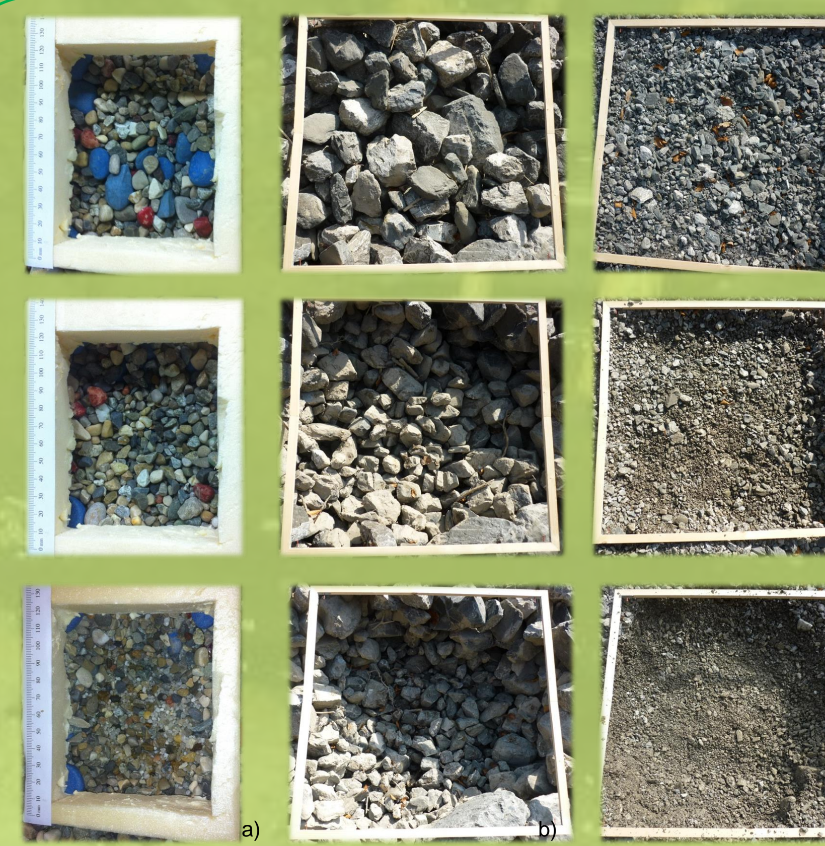
Vertical grain size sorting on deposit: a) in small scale experiment and b & c) in the field
