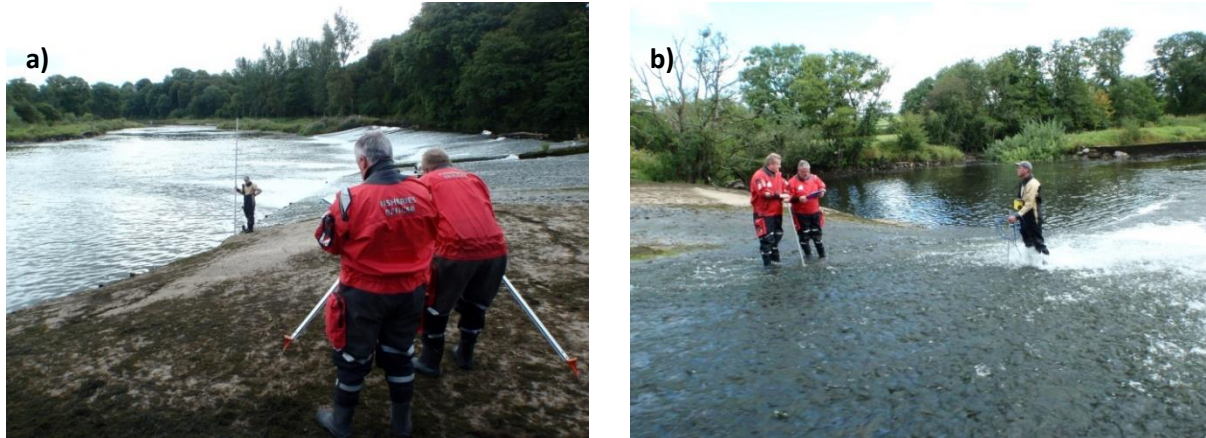
Figure 4.22. SNIFFER survey at a barrier to salmon, sea lamprey and shad in River Munster Blackwater: a) taking levels and b) taking velocity readings.
