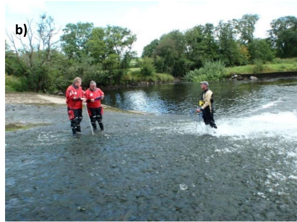
Figure 4.22. SNIFFER survey at a barrier to salmon, sea lamprey and shad in River Munster Blackwater: a) taking levels and b) taking velocity readings.
