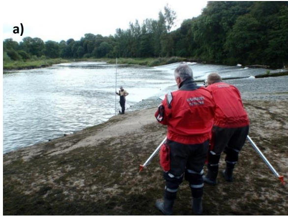
Figure 4.22. SNIFFER survey at a barrier to salmon, sea lamprey and shad in River Munster Blackwater: a) taking levels and b) taking velocity readings.
