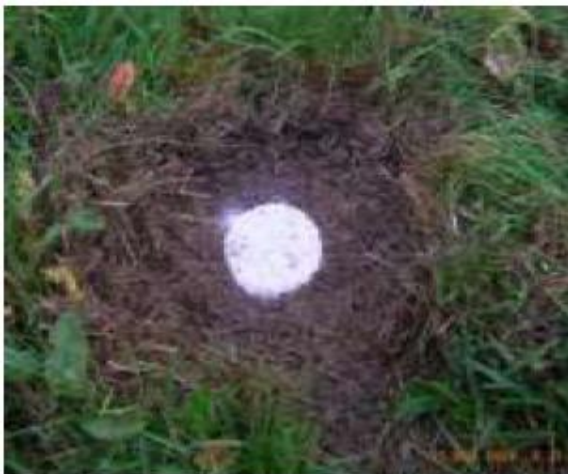
Figure 2-2: Setting up the sand layer. On the left, a layer of several mm thickness. On the right, a minimum thickness layer, but which probably extends too much beyond the cylinder.
