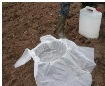
Figure 2-3: Photos of the Beerkan experimental protocol. Left: undisturbed soil sampling to get initial soil moisture and dry bulk density. Middle: Filling of the cylinder with the plastic sheet before starting the infiltration test. Right: Measurement of the water level during infiltration.
