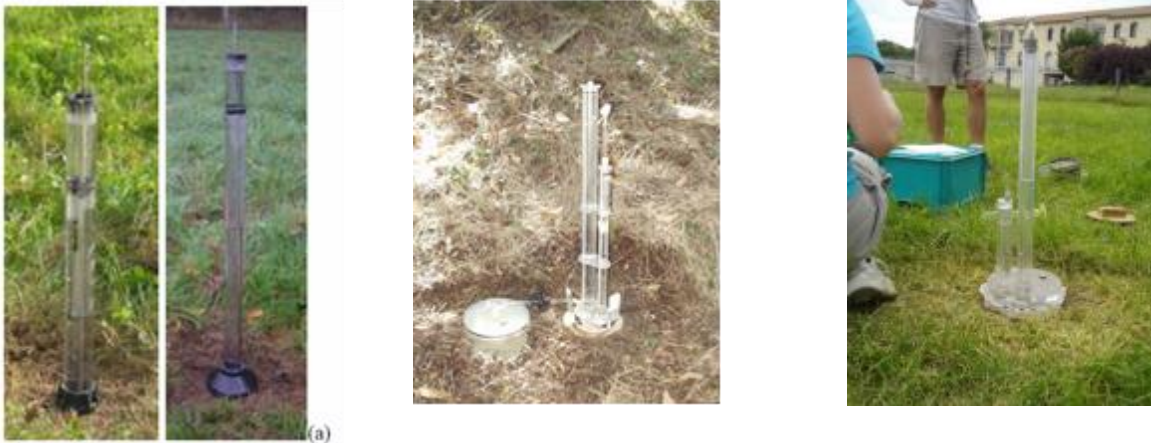
Figure 2-1 : (a) Photo of mini-disk infiltrimeters (4.5 et 8 cm in diameter) (Photo Irstea) ; (b) Infiltrimeter where the disk was removed from the tower from HSM (Photo C. Bouvier) ; (c) Infiltrimeter used at LTHE (Photo I. Braud)
