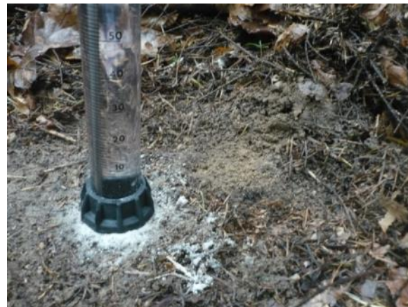
Figure 2-2: Setting up the sand layer. On the left, a layer of several mm thickness. On the right, a minimum thickness layer, but which probably extends too much beyond the cylinder.
