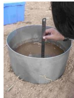
Figure 2-3: Photos of the Beerkan experimental protocol. Left: undisturbed soil sampling to get initial soil moisture and dry bulk density. Middle: Filling of the cylinder with the plastic sheet before starting the infiltration test. Right: Measurement of the water level during infiltration.
