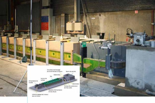
The possibilities for development of a new lock, preventing salt water from penetrating into the fresh water reservoir, was studied. A scientific model has allowed to verify the technical data in this innovative project.
