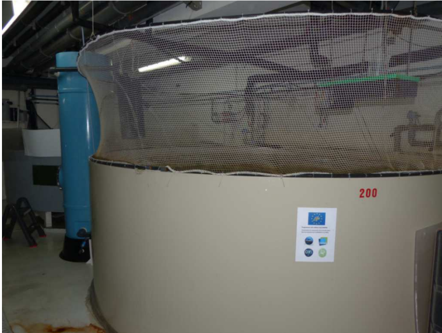
Figure 4 : The 9.3 m 3 rearing tank with the final net system to prevent escapements.
