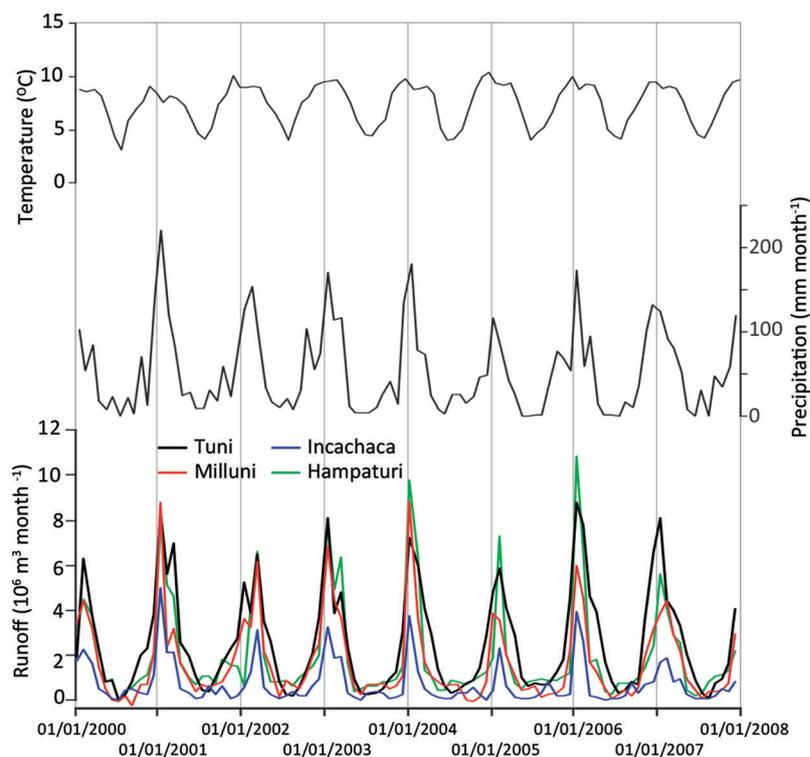
**Fig. 2.** Monthly runoff from La Paz drainage basins, monthly mean precipitation measured at San Calixto and El Alto weather stations and monthly mean temperature measured at El Alto station over the period 2000–07.
