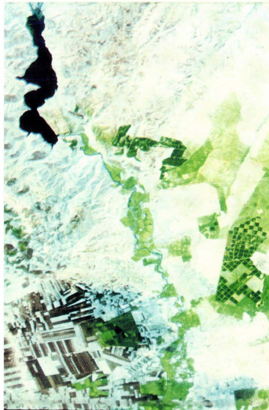
Figure 6. Landsat TM image of 10 July 1987 showing areas irrigated by private pumping units (in green along the river)
