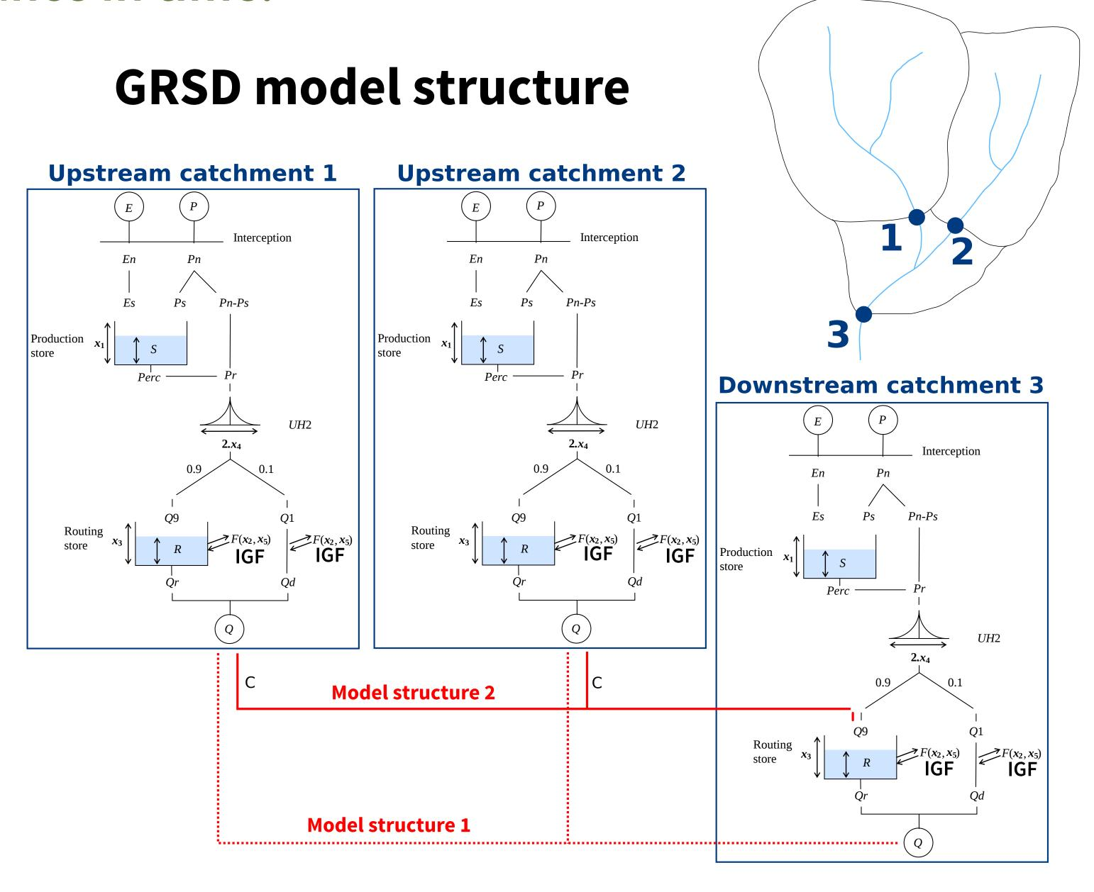
The semi-distributed model GRSD is based on an implementation of a lumped daily GR5J model (5 parameters) on each subcatchment. GR5J is composed of two stores: a production store (capacity *X1*) and a routing store (capacity *X3*), which is filled by the output of a unit hydrograph (of time base *X4*). Two other parameters, *X2* and *X5*, are used to quantify the IGF. Outflow simulations of upstream catchments are routed downstream using a streamflow celerity (parameter *C*).
