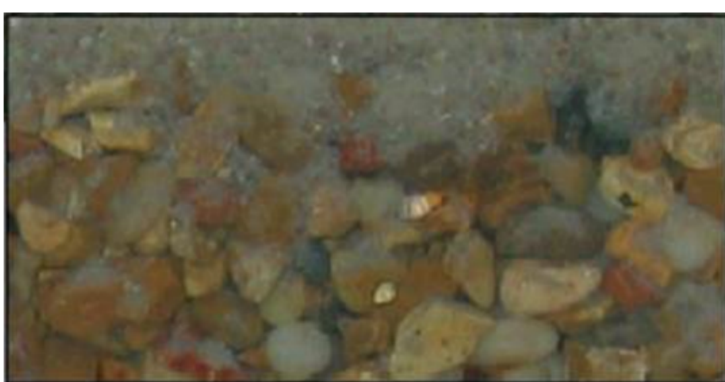
Sealing process: clogged layer at bed surface [2]
