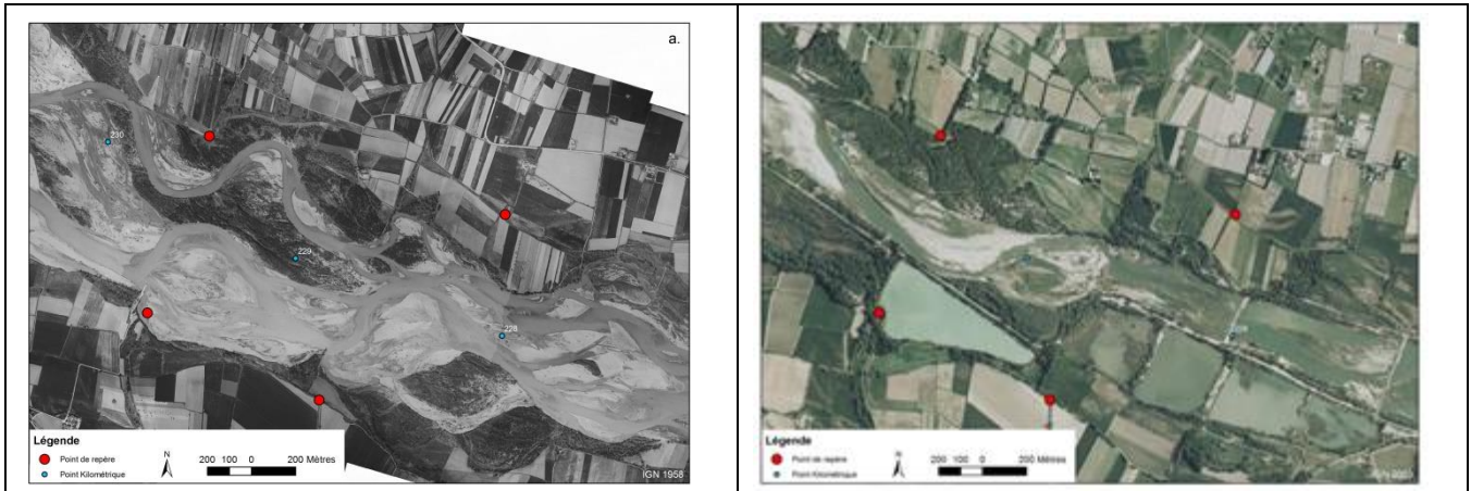
Figure 14: Changes to the Durance bed between 1958 and 1998, associated with sediment extraction and the construction of the Serre Ponçon dam. (Based on Chapuis and Collomb, 2012) 19 .
