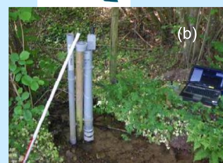
Figure 2: a) soil moisture and (b) water level sensors in the field
