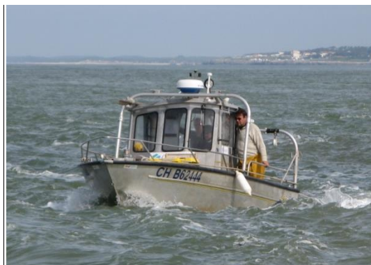
Figure 3 : Dedious , coque en aluminium, 7m de long.
