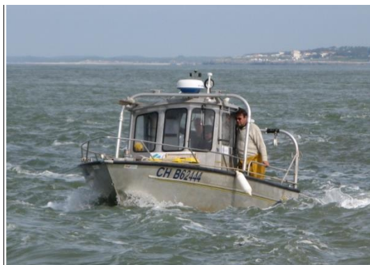
Figure 3 : Dedious , coque en aluminium, 7m de long.
