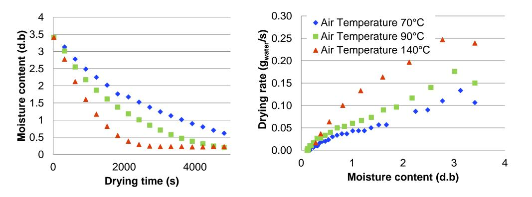
After a period of adaptation, the curves exhibit a narrow plateau, which is quickly followed by a long falling rate zone. Pure internal transfer limitations appear for a moisture content close to 0.7 (d.b.).
