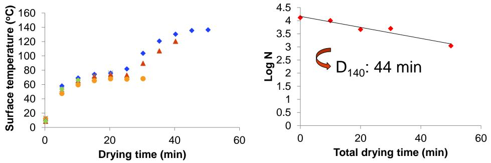
At 140°C for 44 minutes, drying induces a reduction in the concentration of *C. perfringens* by 1  $\log_{10}$  unit. At 70°C, the same fall in concentration is achieved after 128 minutes.
