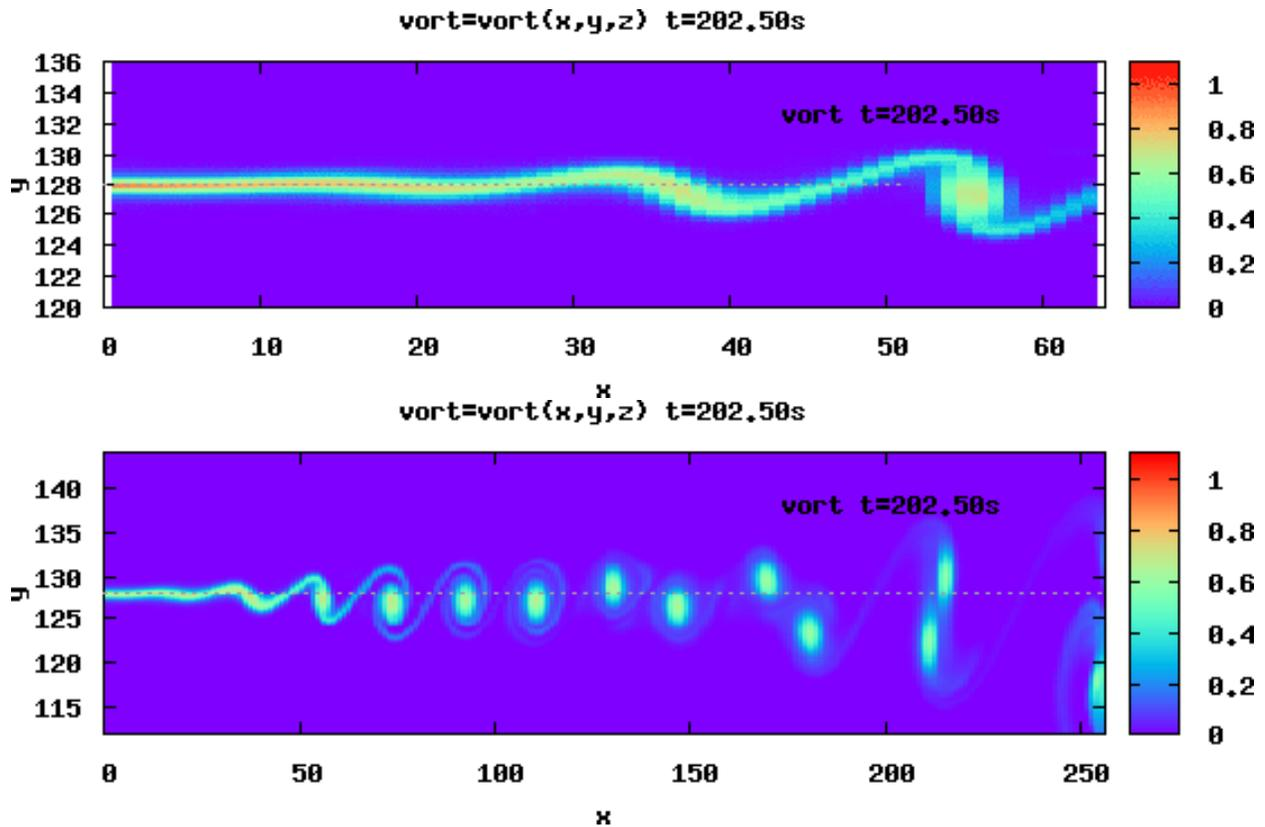
Figure 2. Instantaneous vorticity maps in the model plant in presence of permanent disturbances and without control after 202s of simulation: on top, a zoom on the region of interest; on bottom, the whole map.
