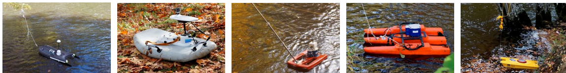
Figure 2.3: ADCPs and associated tethered boats (from left to right: M9 mounted on HydroBoard, M9 on TorrentBoard, StreamPro on Small Catamaran, StreamPro on Catamaran and Q-Liner).
