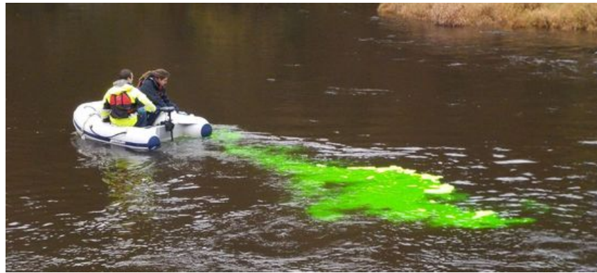
Figure 2.13: Dye dilution gauging downstream of the dam (Source: A. Despax).
